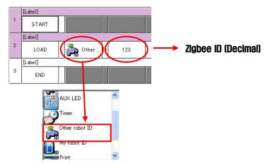
Once other Zigbee's ID set, it is maintained even after power is turned off. As other ID is used for simple communication, the ID can be changed accordingly by users.
