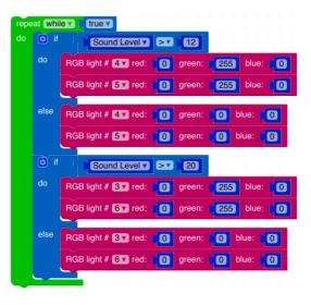
Note the commands used in the 'else' section. These are used to ensure the lights switch off again rather than switching on and staying on.
