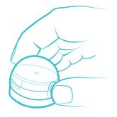
Hold down the power button on Ozobot for 2 seconds until the LED light turns white. 2
