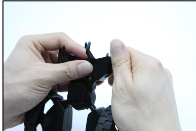
2) Hold the wing bracket with one hand And hold the horizontal wing to separate.
