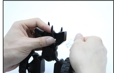
3) Remove the horizontal wings by twisting the hand forward.
