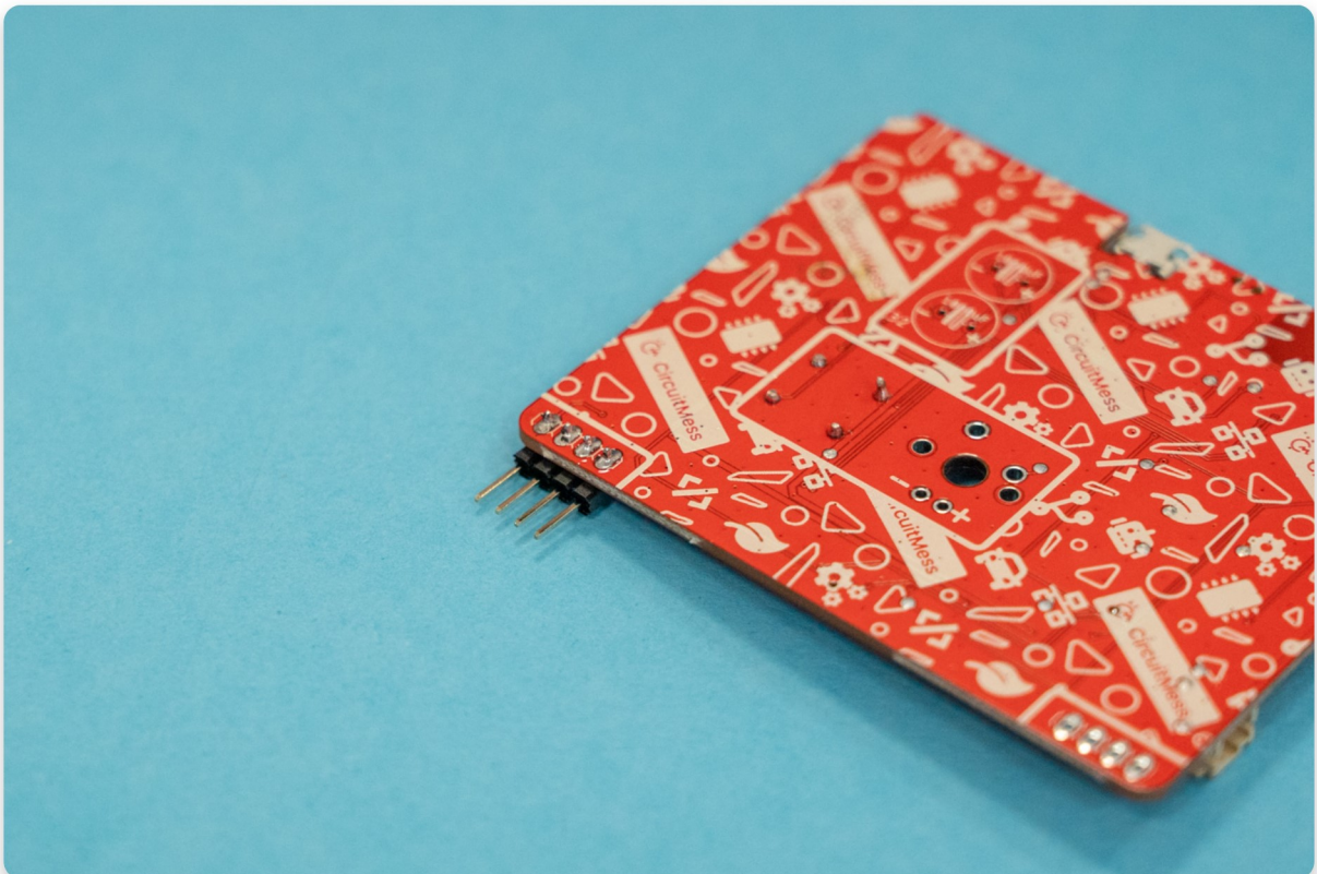
The first pin header soldered to the board
