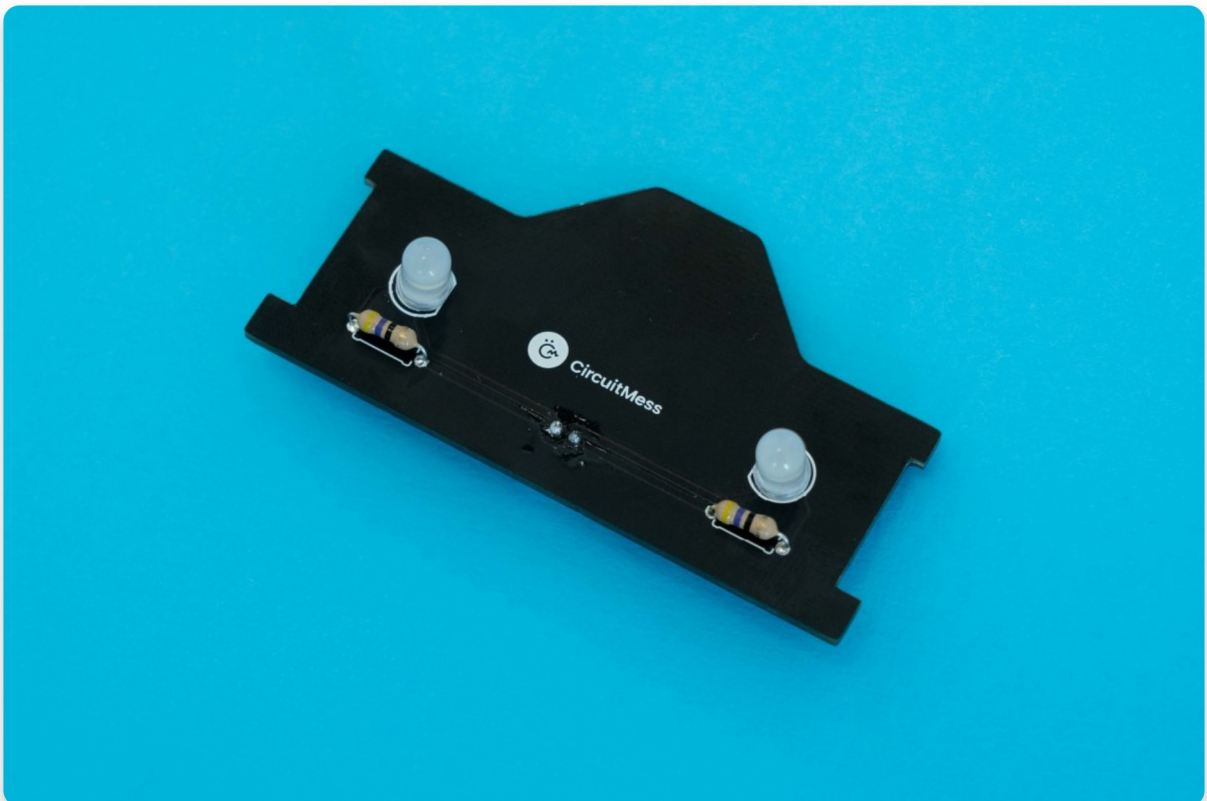
LEDs soldered to the board
