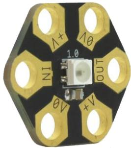
The design of the ZIP HEX makes it possible to stack them by rotating the PCB 180 degrees to create columns.
