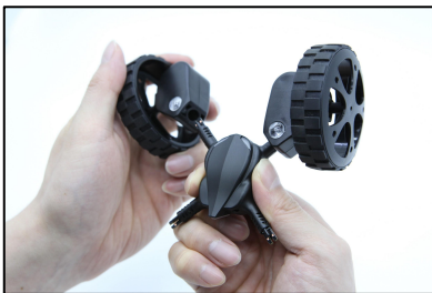
4) Insert the drive-only motor bracket to the front of Petrone Body.
