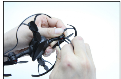
3) Hold the motor bracket and pull the propeller separator.
