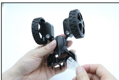
7) Assemble the horizontal wings on the wing brackets on both sides.
