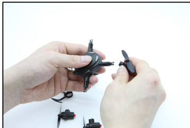
2) Remove the Motor Bracket from the Petrone body.
