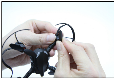
5) Insert the propeller to fit in the motor bracket.
