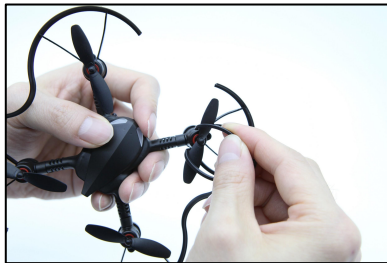
2) Hang the propeller separator to the propeller
