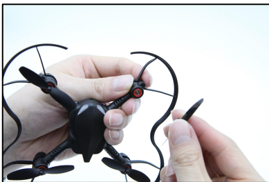
4) Check the direction of rotation of the propeller to replace.
