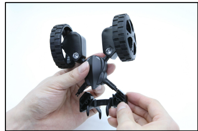
6) Insert the assembled wing Bracket to the rear of Petrone Body
