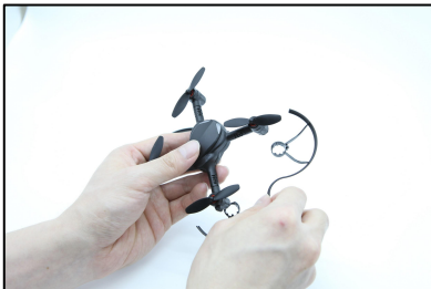
1) Remove the propeller guard from the Petrone body.
