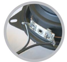
Take the cable connected to one speaker and connect it to the terminal block labeled 'OUT1' on the PCB. The connections on the terminal blocks are also labeled with a '+' and '-'. The '+' on the PCB needs to go to the '+' on the speaker and '-' to '-'.
