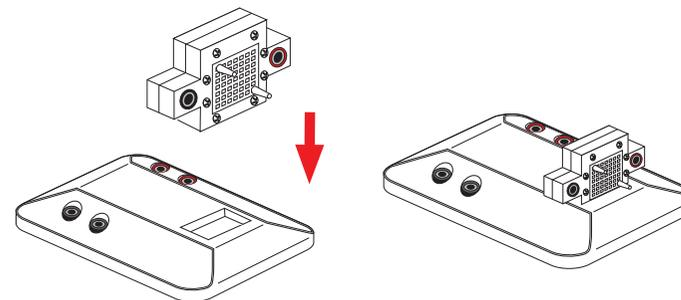
b. Use the short black & red wires to connect the fuel cell to its base as shown below. Make sure you respect the color code when you plug each wire into the corresponding socket.
