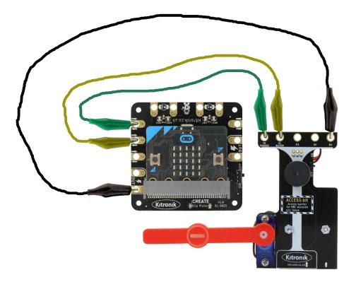
Connect crocodile clip leads between the Pin 0 output on the Klip Motor board and P0 on the ACCESS:bit, the Pin 1 output on the Klip Motor board and P1 on the ACCESS:bit, the 3V output on the Klip Motor board and the 3V connection on the ACCESS:bit, and finally the GND connection on the Klip Motor board and the GND connection on the ACCESS:bit.
