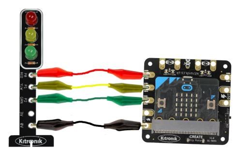
Connect crocodile clip leads between the Pin 0 output on the Klip Motor board and P0 on the STOP:bit, the Pin 1 output on the Klip Motor board and P1 on the STOP:bit, the Pin 2 output on the Klip Motor board and P2 on the STOP:bit, and finally the GND connection on the Klip Motor board and the GND connection on the STOP:bit.
