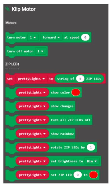
Within the extension, the blocks are split by motor control and ZIP LED control. A short description of the function of each block is given in the table below:
