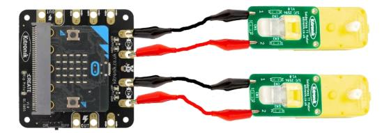
Connect crocodile clip leads between the motor outputs on the Klip Motor board (one pair labelled M1 and the other labelled M2), and the exposed pads on the solderless motor attachment boards.
