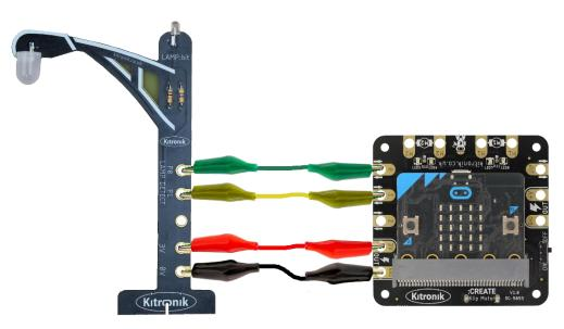
Connect crocodile clip leads between the Pin 0 output on the Klip Motor board and P0 on the LAMP:bit, the Pin 1 output on the Klip Motor board and P1 on the LAMP:bit, the 3V output on the Klip Motor board and the 3V connection on the LAMP:bit, and finally the GND connection on the Klip Motor board and the GND connection on the LAMP:bit.
