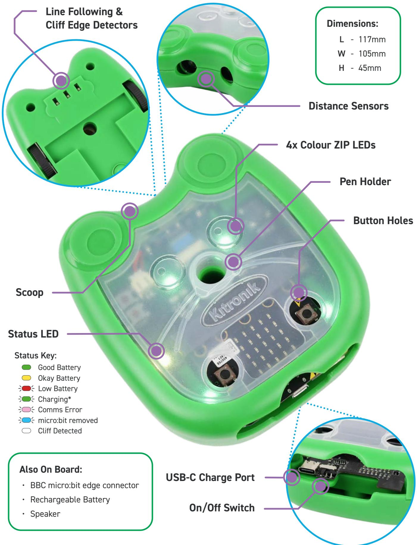
\* Mai-Z will charge both while switched on and switched off. While on, the Status LED indicated here will show. While off, a separate LED will indicate red while charging, and green when charged.
