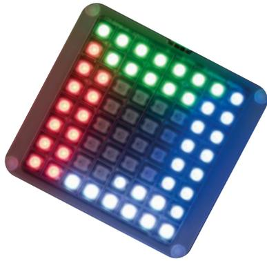
Switching the pixel off after each step makes it appear to move.
