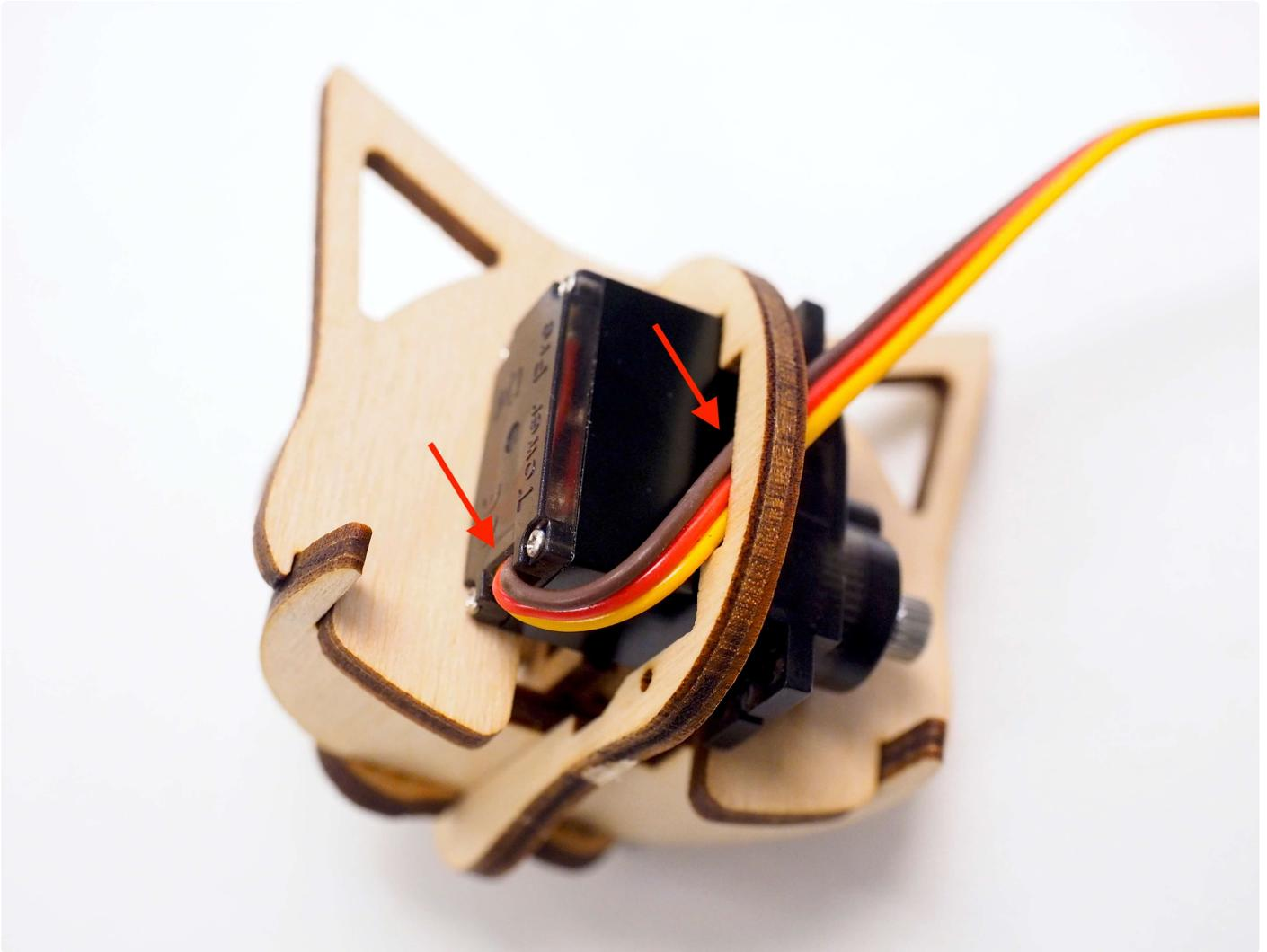
⚠ DO NOT connect the head with the neck yet, because the tilt servo on the head has to be calibrated.
