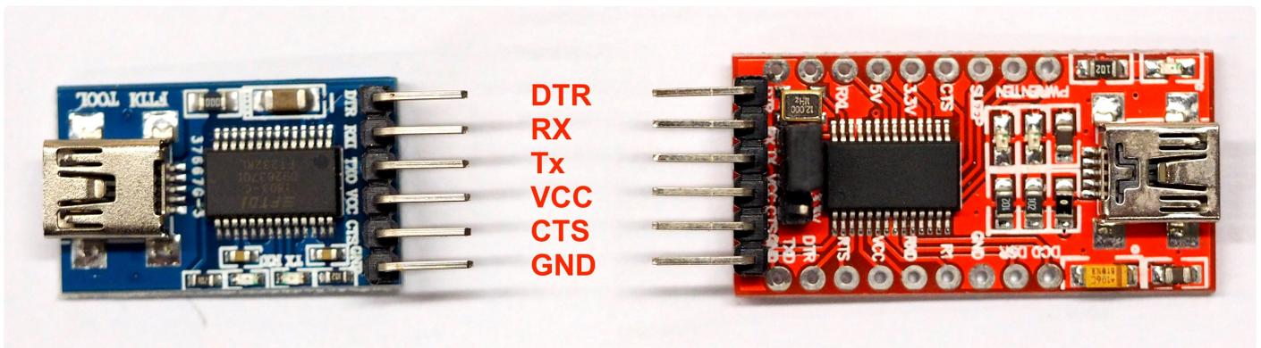
On the red board, the jumper selector should be put on 5V (not 3.3V) on the uploader for Arduino. Match the GND on both the uploader and the 6-pin socket on NyBoard.
