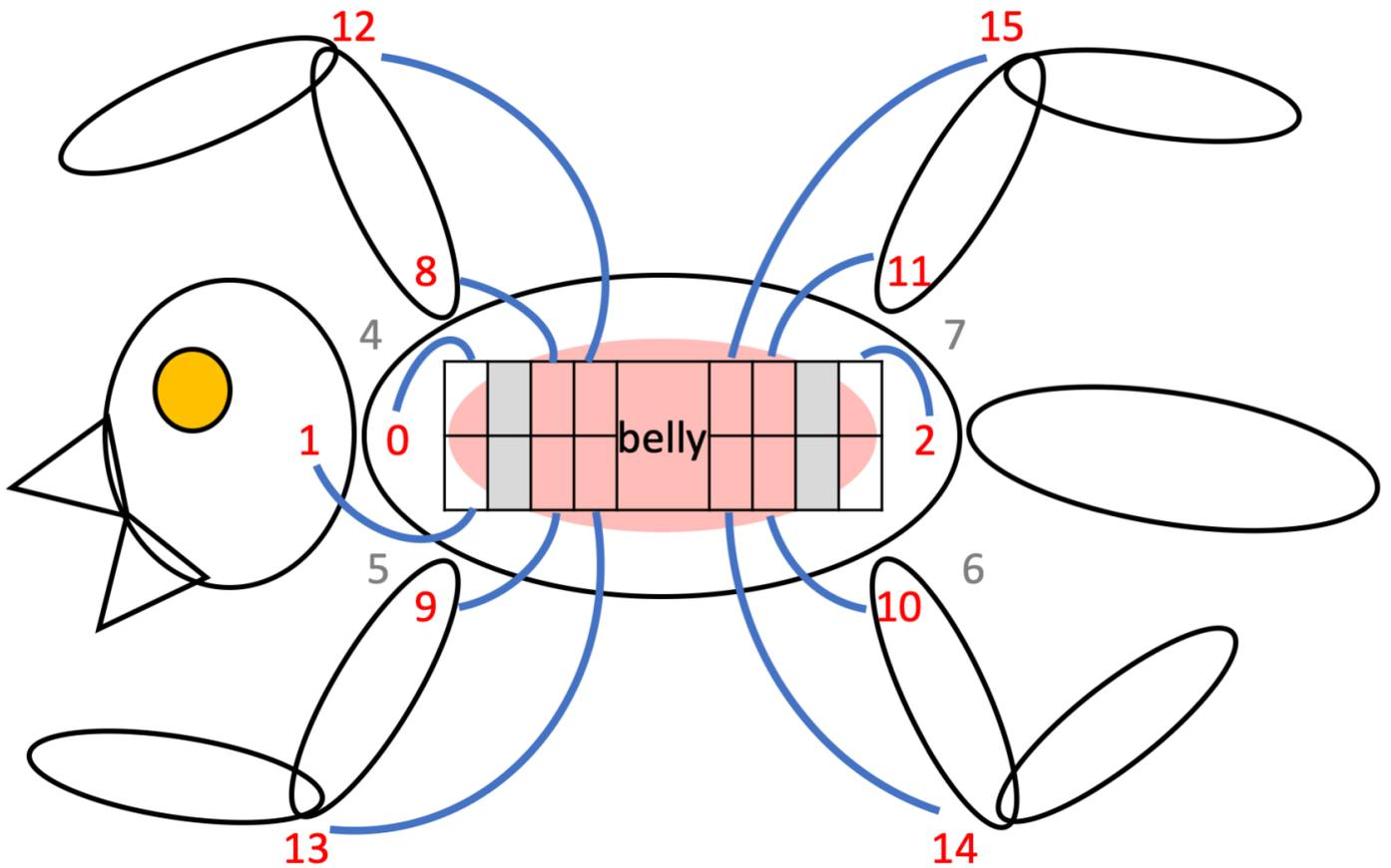
**i** NyBoard V0\_\* and V1\_\* have different PWM pin orders, but the physical servo connection remains the same. All adjustments are handled in the software. **You don't even need to read the pin numbers on the PCB board.**
