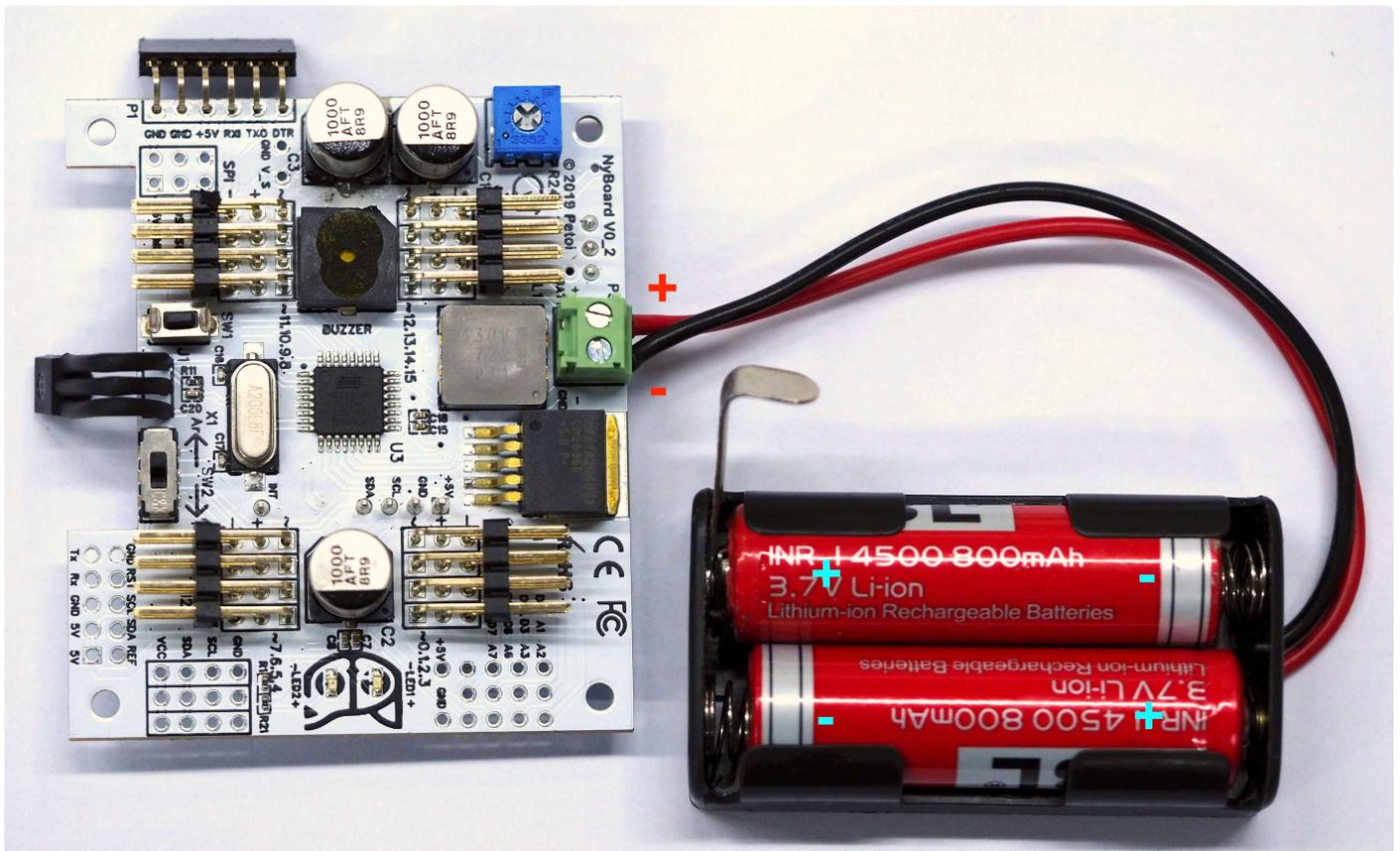
In the kit shipped after Jan.1st, the terminal is replaced with an anti-reverse socket, so you won't be able to
