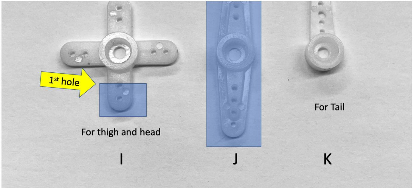
**i** In kits after January 2021, we included the new servo arms that requires minimal efforts to cut. You only need to cut the cross-shaped servo arm to make the L-shaped connector for the neck joint.
