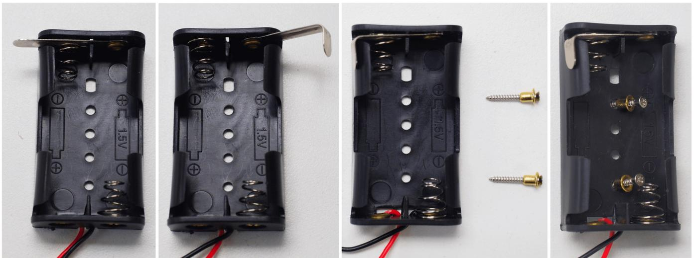
The spring attached structure of the battery holder is used for shifting the center of mass when fine-tuning gaits.
