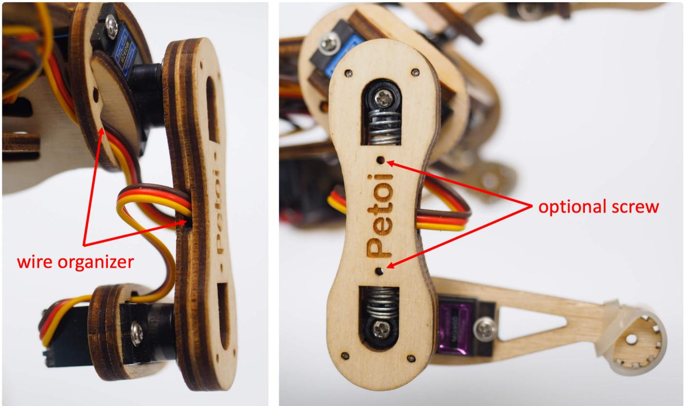
The servo arm should be able to slide in the track on thigh2 with subtle friction after thigh1 and thigh2 are screwed together. You can tune the tightness of screw C to achieve proper friction. If you need more control over the tightness:
