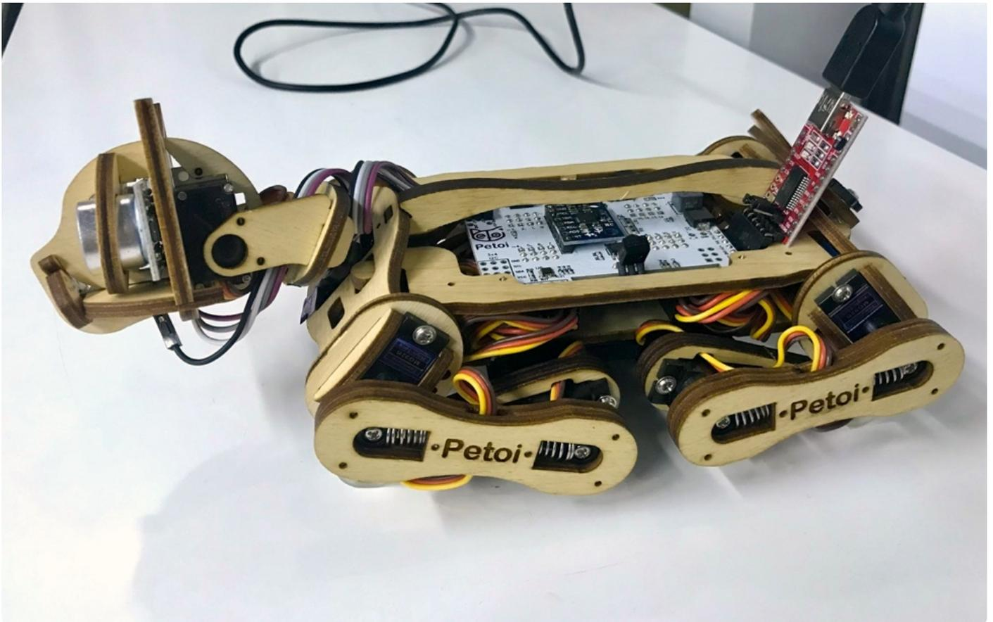
Connect your computer with the FTDI uploader (the red chip with 6 male pins) through mini-USB to USB cable. The uploader has three LEDs, power, Tx, and Rx. Right after the connection, the Tx and Rx should blink for one second indicating initial communication, then dim. Only the power LED should keep lighting up. You can find a new port under **Tool->Port** as `/dev/cu.usbserial-xxxxxxx` (Mac) or `COM#` (Windows).
