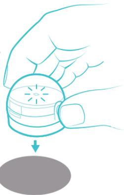
Release the power button and set Ozobot in the middle of the black dot (included in the Activity Set) while the LED light is flashing white.
