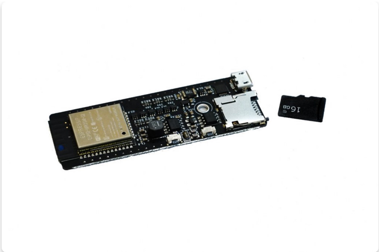
The brain board and the SD card
