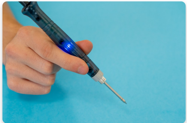
The blue light means that the soldering iron is turned on
