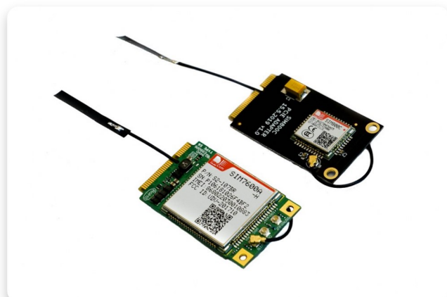
Both SIM7600 (4G) and SIM800 (2G) boards
