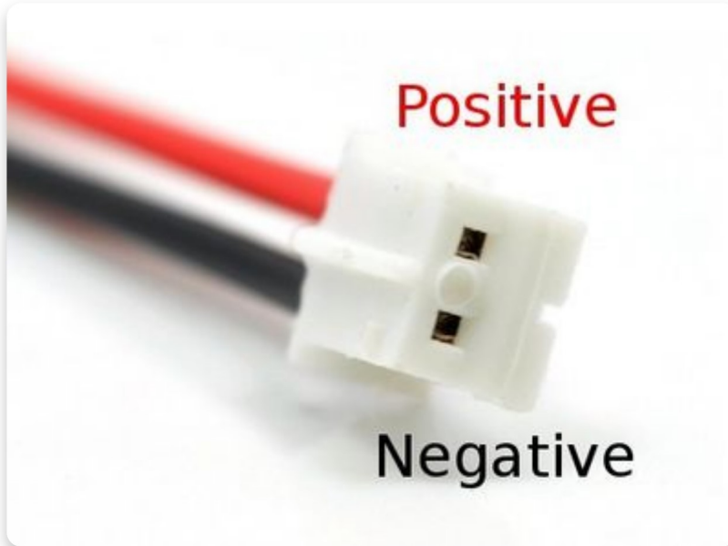
JST cable that connects the battery
