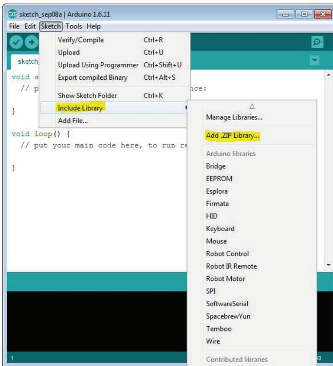
After the library is installed, close and restart the Arduino Software (IDE). After it's restarted, you can access the coding examples by selecting **Examples** under the File menu and scrolling down to the TETRIX\_Tele-Op library.
