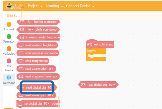
Figure 2.3.2 read digital pin P0 block
