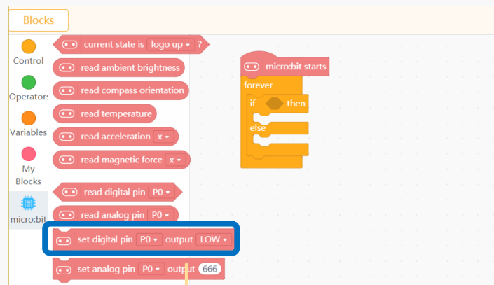
Figure 3.1.5 “set digital pin output”
