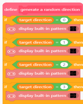
Figure 4.4.4 "generate a random direction" function
