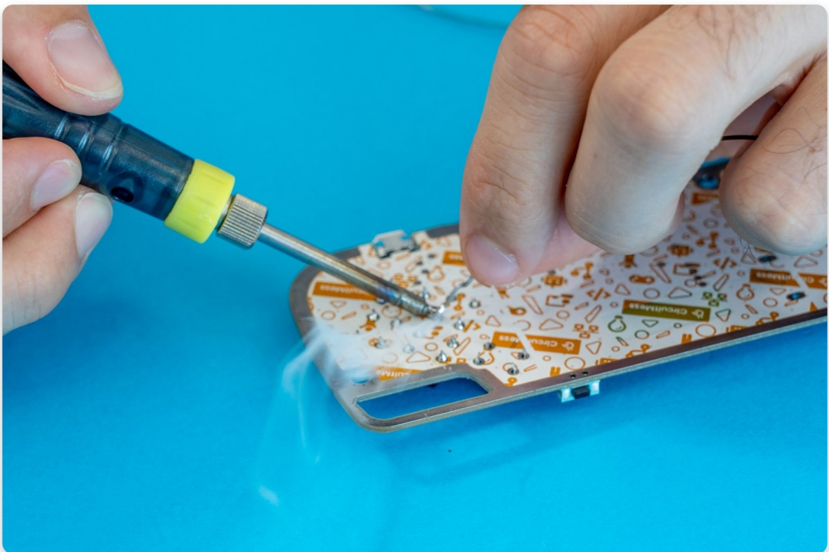
Soldering the rest of the buttons
