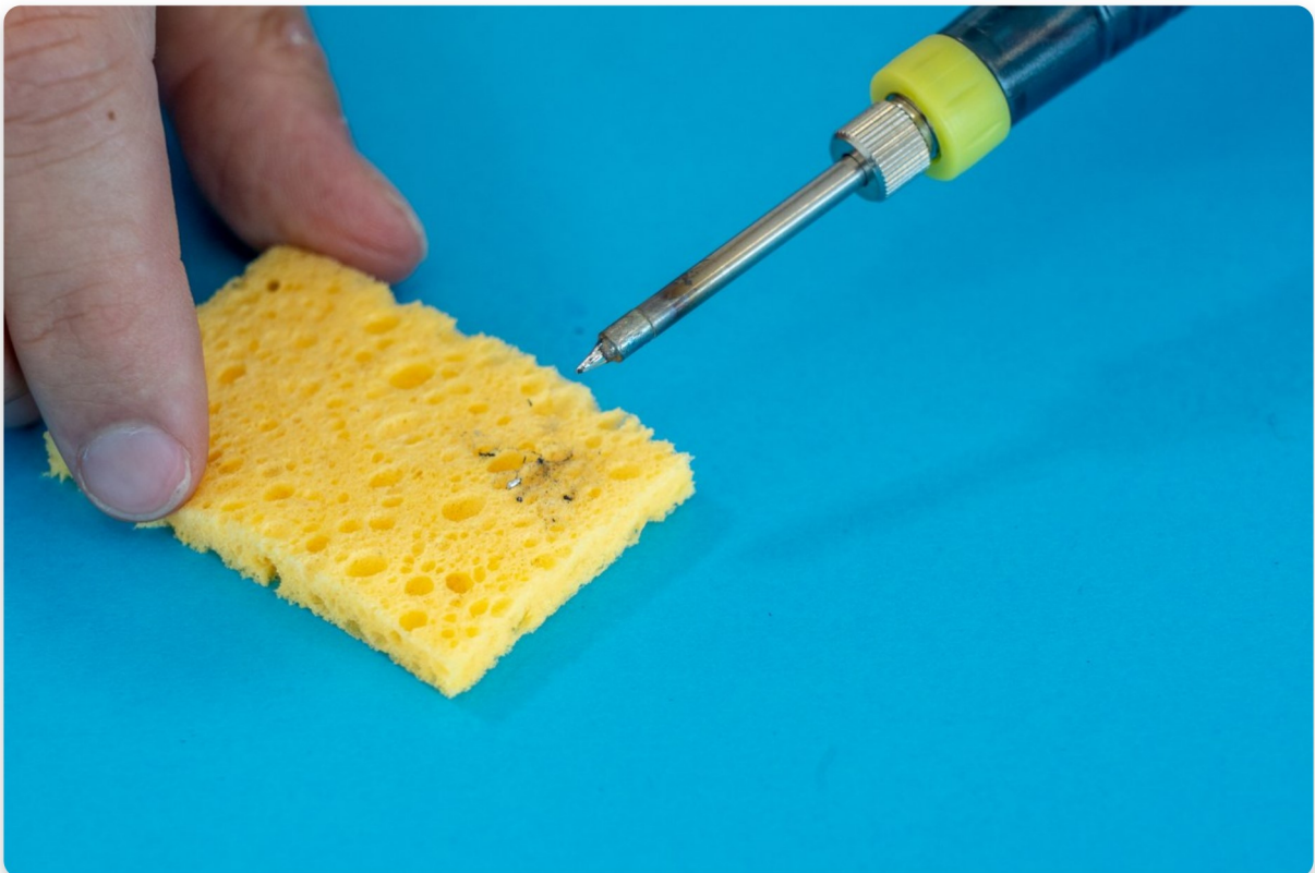
Cleaning the tip of the soldering iron
