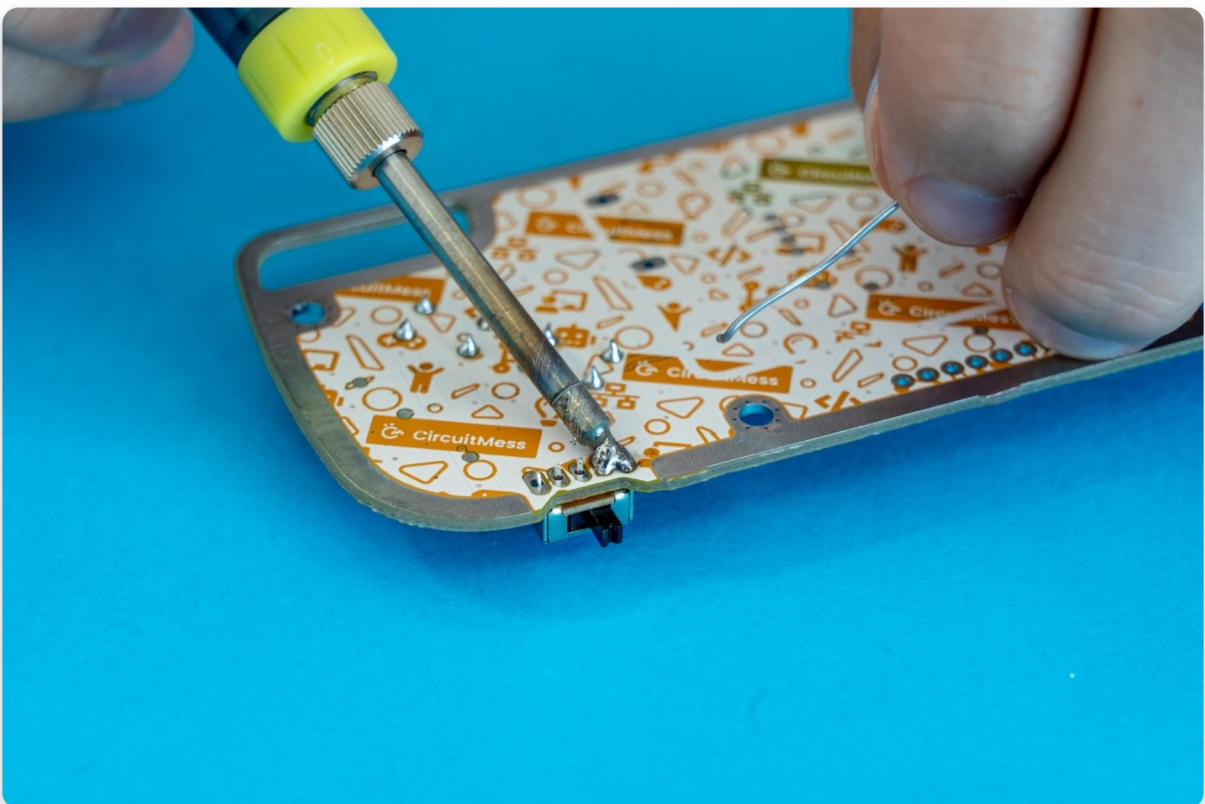
Example of a solder bridge
