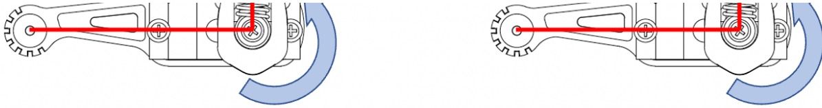
A visualization of the perfect zero(calibrated) state when you enter the calibration mode
