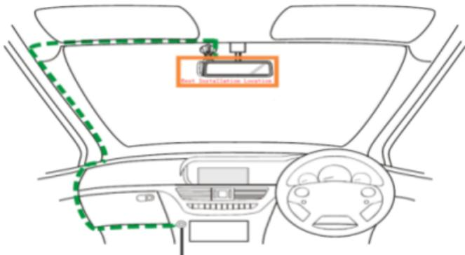
*The above illustration refers to a right-hand drive car. For left-hand drive cars, please flip the position of the cable installation accordingly.*
