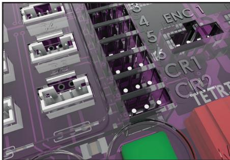
Figure 31: PRIZM Continuous Rotation (CR) Servo Motor Ports
