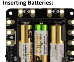
The Klip Motor Driver requires 3 x AA batteries to provide power to the connected BBC micro:bit and any extra attached devices. These are shown inserted in the correct orientation in the image to the left.
