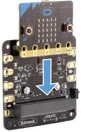
The BBC micro:bit needs to be firmly inserted into the edge connector with the BBC micro:bit LEDs visible to the user.
