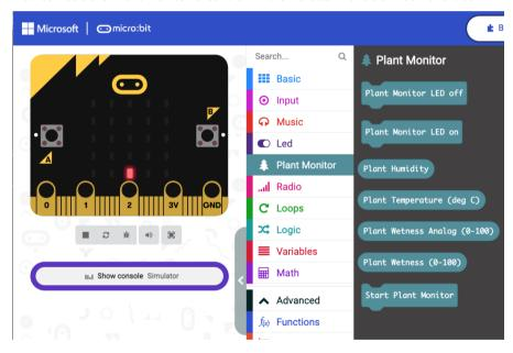
As well as the Start Plant Monitor, Plant Humidity and Plant Temperature blocks, there are also blocks that turn the LED on and off.
