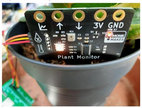
The front side of the prong should be as close to the edge of the pot as possible. The sensing all takes place from the far side of the prong.
