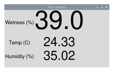
Try holding the prong of the moisture meter and you should see the wetness % rise. Similarly putting your finger over the metal box on the Plant Monitor that is the temperature and humidity sensor will change both readings.
