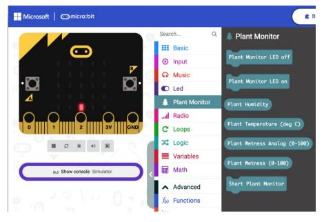
As well as the Start Plant Monitor, Plant Humidity and Plant Temperature blocks, there are also blocks that turn the LED on and off.
