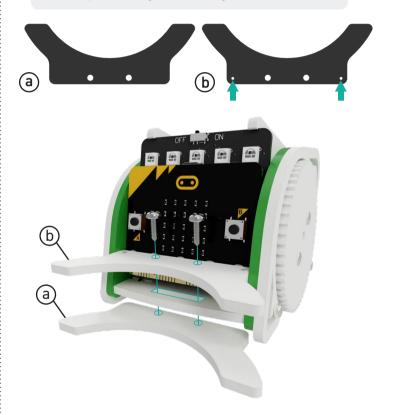
**NOTE:** The screws self tap into the holes on the lower panel.
