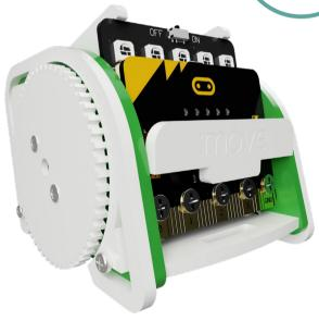
Using the screws provided, screw the two panels either side of the :MOVE mini baseplate. The screws should pass through the rectangular cut-out.
