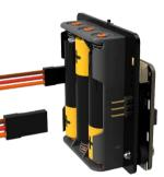
**STEP 1:** Plug the servo cables back into the Servo:Lite board. The left servo should plug into the left-hand side of the board and vice versa. The cables should be threaded down the gaps on either side as shown below.
