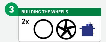
**STEP 1:** Stretch the 0-Ring round the wheel, this will act as a tyre for :MOVE mini. Press fit the wheel onto the servo shaft and repeat for the opposite side
