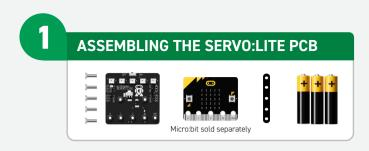
**STEP 1:** Use a small Phillips screwdriver to screw the five M3 machine screws through the micro:bit and spacer into the nuts mounted on the PCB.
